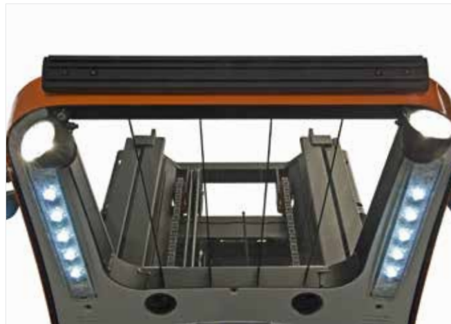
Integrated LED lights in the overhead guard enhance comfort and safety during operations.
