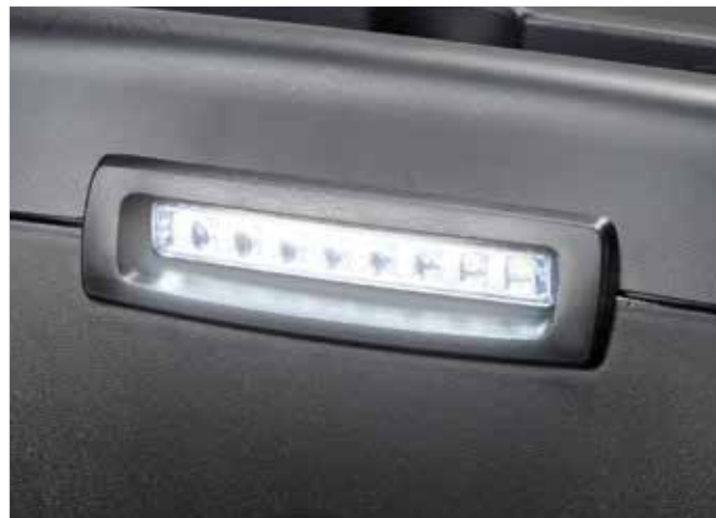
LED front light raises the awareness of the truck in busy environments and enhance safety in the warehouse.
