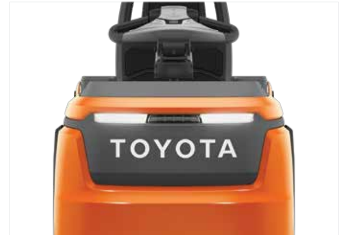
Optional integrated daytime running lights and blue/red warning lights enhance safety in the warehouse.
