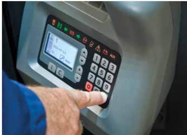
Access Control prevents unauthorised use and preset each driver's personal parameters upon start-up.
