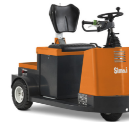
The 3-tonnes compact model TTE30 allows the driver to stand or sit for longer travel distances or to stand for quicker on/off.
