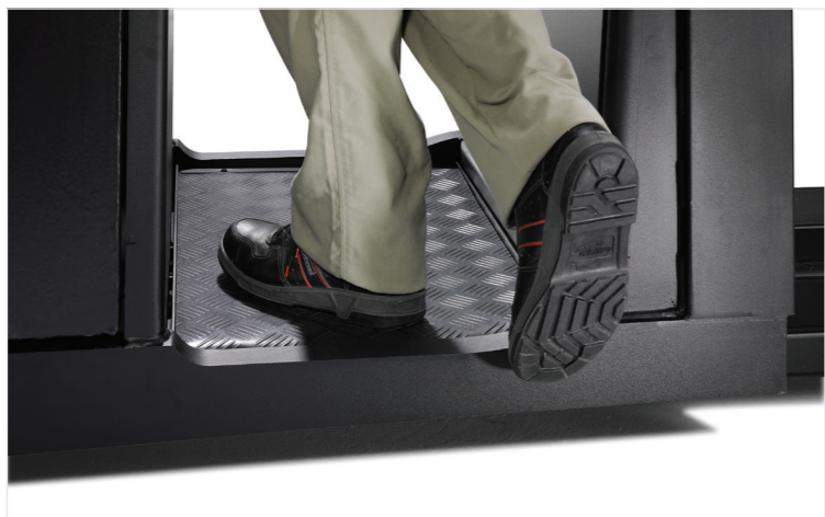
Low step-in and optional vibration-damped floor.
