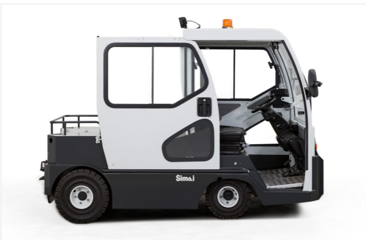
Steel cabin with sliding doors as option available for easy on and off.
