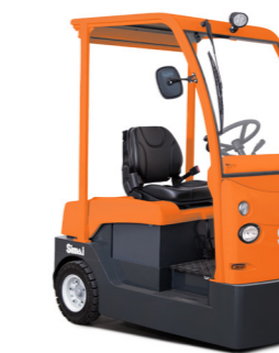
The TTE71 has a towing capacity up to 7 tonnes, built to transport heavy loads for production or other applications.
