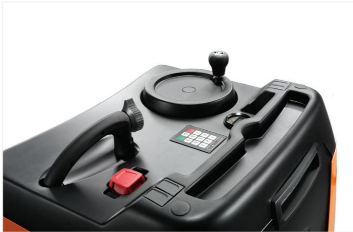
'Spinner wheel' steering and PIN-code access.
