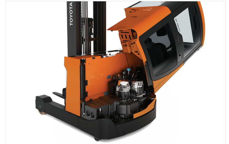
Easy access to motor compartment for efficient maintenance.
