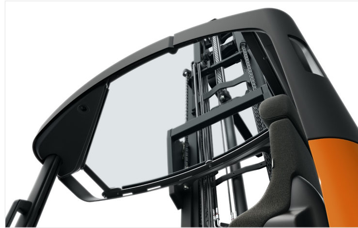
The transparent overhead guard is designed to give the best possible protection for the driver without compromising on visibility when working at height.
