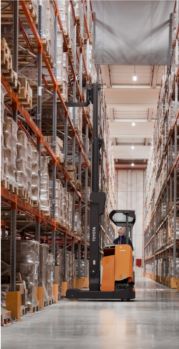
The transparent overhead guard is designed to give the best possible protection for the driver without compromising on visibility when working at height.
