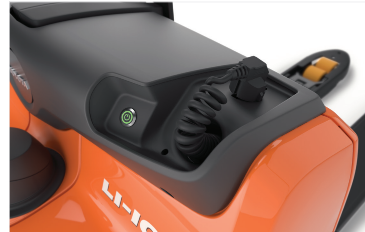
Easy and fast charging with the built-in charger for more energy efficiency (external charger also available).
