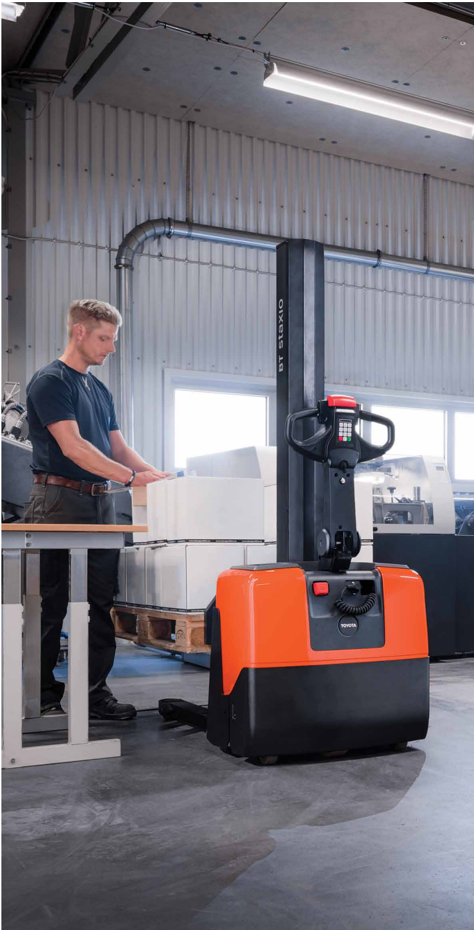
HWE100S model can handle a variety of pallet sizes thanks to its adjustable straddle forks
